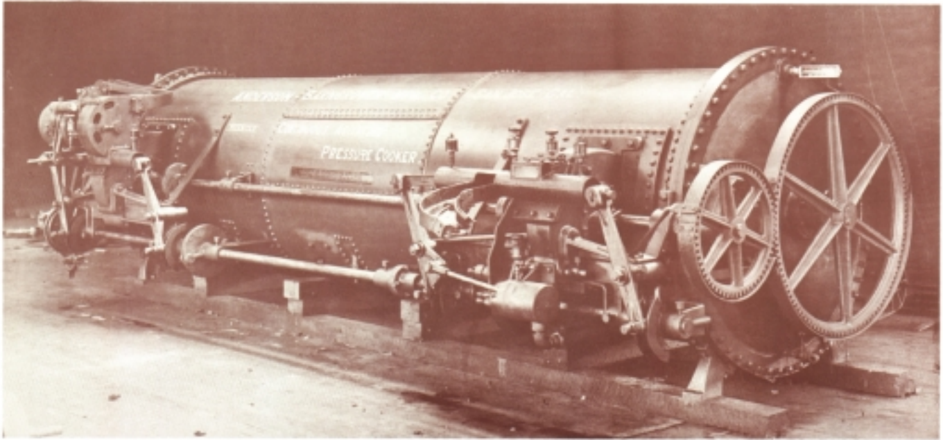
IN 1915, this pressure vessel was introduced. It's sliding valves were too slow, and it was re-designed.
