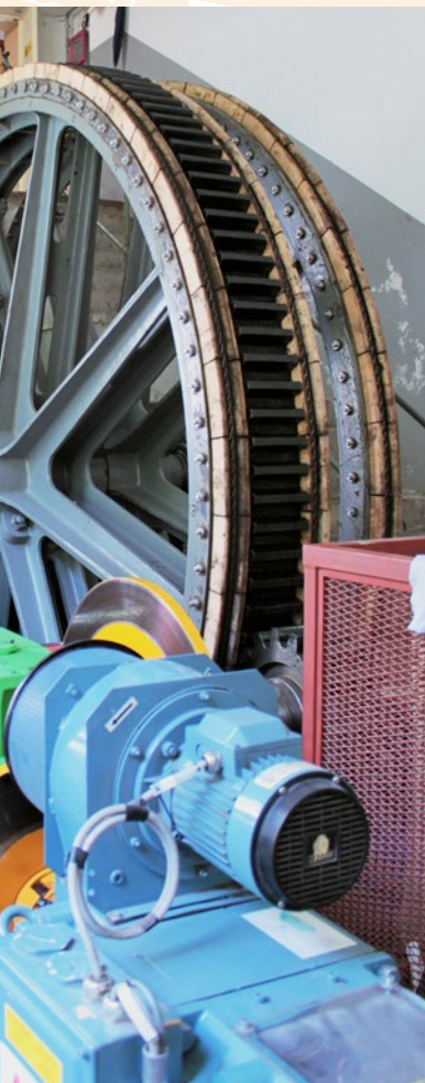
Figure 5: The drive gear used since 1912 in the engine building at the top station. The three cable driving grooves on the large diameter wheel are made out of wood. They form a total deflection angle of more than 3 times 180 degrees (to be applied in the belt friction equation). At the bottom partly visible is the blue electric drive motor, from the intermediate gear only the green corner is visible. Both are from the 1998 restoration.
