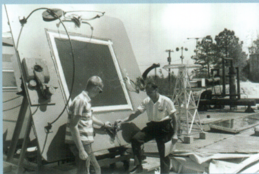
Prof. Erich Farber (r) adjusting the ASHRAE/UF calorimeter, with an early SEECL student (mid 1950s).
