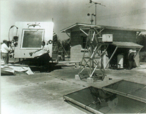
Prof. Erich Farber (r) making adjustments to the ASHRAE/UF calorimeter, at the early SEECL experimental pad, at the Gainesville Regional Airport (mid 1950s).
