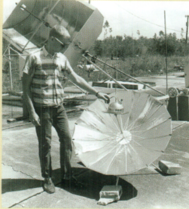
Early SEECL student demonstrates solar cooking on a collapsible umbrella cooker. The concentrated solar radiation heated the teapot water quite effectively -- and the collapsing umbrella made storage easy (mid 1950s).
