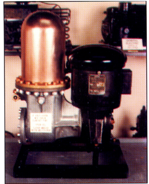
Nizer Compressor and Water Cooled Condenser for Ice Cream Cabinets. (1923 - 1925)
