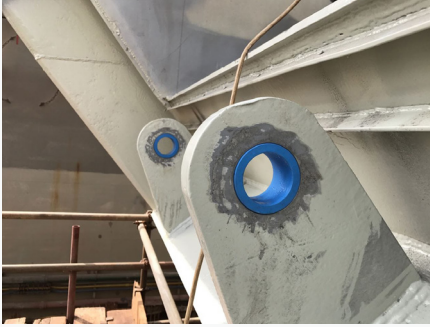
Grease-free ThorPlas-Blue bearings installed on a Landing Craft Utility vessel
